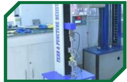
TEAR AND PUNCTURE RESISTANCE TEST
